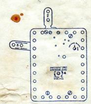
Before commencing to wind up the motor, move the brake-lever 2 over to the right. To wind, press the key down on to the winding-spindle 4 as far as it will go, and turn it in the direction of the arrows. Never turn the key backwards. To start the motor, release the brake-lever.
