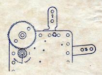
The motor with drive a large number of the smaller models without extra gearing. This diagram shows how extra gears may be added when more power is required. The wheel mounted on the driving-spindle is the  $\frac{1}{2}$ " Meccano pinion; the wheel engaged by the pinion is the Meccano 56 toothed gear.
