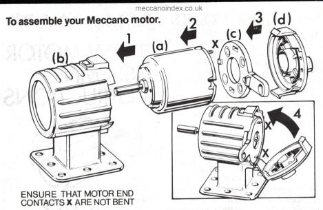
Position motor (a) in motor housing (b) with end contacts at top and bottom (see inset). Locate the switch lever (c) (smooth side outwards) over the motor end contacts. Hold the motor end cap (d) with 'Meccano' upwards. Insert the lower locating lugs then position top locating lug and push until it 'clicks' home.
