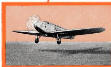
A well-known German single-engined commercial low wing monoplane is the Junkers F.13L, which is a four-seater cabin monoplane equipped with a 280 h.p. Junkers engine. It has a maximum speed at sea level of 123 m.p.h. and cruises at 106 m.p.h. Its tank capacity is sufficient to enable it to travel for a distance of 620 miles without refuelling.
