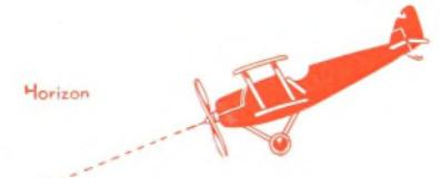
Pushing the stick forward causes the machine to put down its nose and dive.
