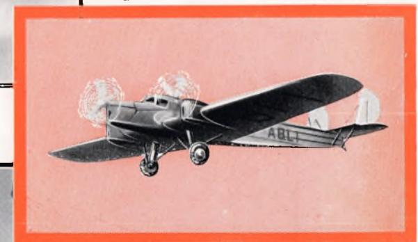
An interesting French triple-engined low wing monoplane is the Dewoitine D-333, which is fitted with three 575 h.p. Hispano-Suiza 9V radial air-cooled engines. This machine accommodates eight passengers, and has two baggage compartments, and separate compartments for the pilots and wireless operators. It can carry a useful load of 3,925 lb.
