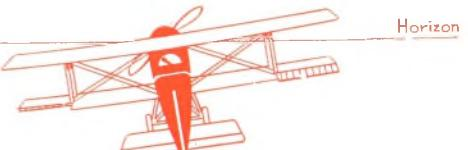
When the stick is moved to the left, the ailerons on that side are raised and the left wings go down, producing left bank.
