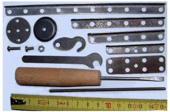
ition a 10h Flat Girder & 2 shorter Threaded Rods can be seen in the models, and in Baukästen. Most of the holes are 3.8mm  $\emptyset$  but those in the Wheel & Pulley Discs, and the centre holes in the 4h long Angle & Flat Girders are 3.0mm. No holes are elongated. The hole pitch is 15.5 mm. The thread is 3mm  $\emptyset$ .
