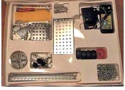
German CONSTRUCTION. All have a bright finish, apart from 4 black Wheels, yellow Windmill Sails, a red Pulley, & a red handled 'electrical' Screwdriver. The exception is a 3\*5h Triangular Plate which looks to have fewer holes than the German part. Also no slotted holes can be seen (apart from in the Face Plate), but this may be the way the parts are lying
